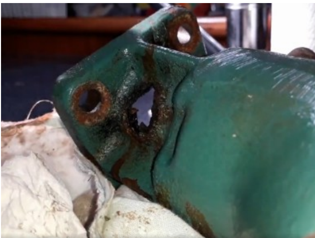
Holes in an old exhaust elbow
